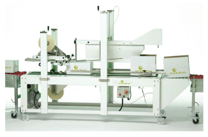
This fully automatic case taper offers outstanding productivity on light cases typically used in the snack food industry. It takes open cases from a conveyor and seals top and bottom using selfadhesive tape.
